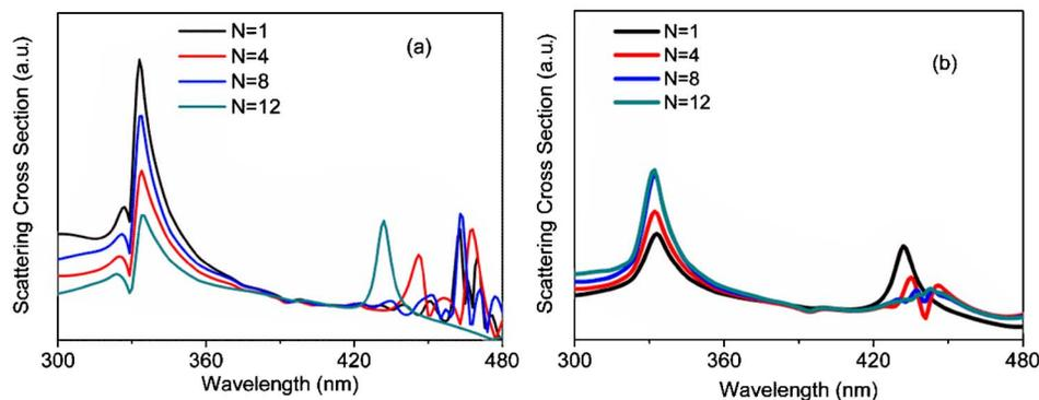
Fig. 3. (Color online) Simulated spectral response of the SCSs for different linear arrays of nanoshell particles ( $r_1=15$  nm,  $r_2=20$  nm) in air. (a) Arrays consisting of 4, 8, and 12 nanoshells spaced by 2 nm; (b) arrays with 4, 8, and 12 nanoshells spaced by 10 nm. A spectrum for a single nanoshell particle is also shown in each panel. Note that for graphic reasons, only the data from 300 nm to 480 nm were displayed in the figures.
