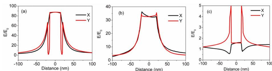
Fig. 7. (Color online) Simulation of the total electric field distribution at resonance, showing the near-field enhancement along the different particle’s cross section. (a) Nanoshell at a resonance wavelength of 539 nm (dipole resonance), (b) solid metallic rod at 341 nm, (c) nanoshell at the multipolar resonance wavelength of 333 nm.
