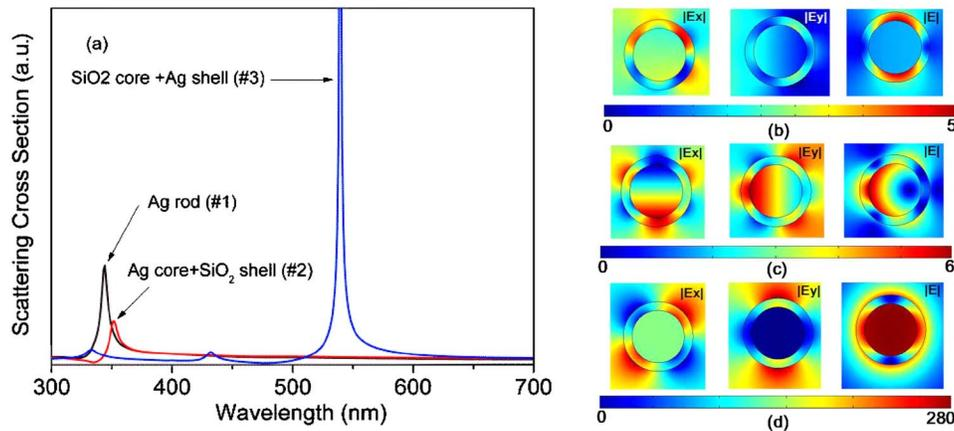
Fig. 2. (Color online) (a) Spectral response of the SCSs of different 2D particle structures; (b)–(d) electric field distributions for the metallic nanoshell (structure #3) with  $r_1=15$  nm and  $r_2=20$  nm [cf. blue curve in (a)] at the three resonance wavelengths (b) 333 nm, (c) 432 nm; and (d) 539 nm. The grayscale bar (color online) shown in the figure quantifies the field enhancement factor, which is defined as the ratio of the obtained maximal field strength to the incident field.
