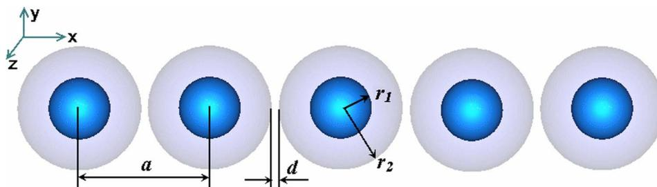
Fig. 1. (Color online) Schematic drawing of a finite nanoshell chain waveguide with constant separation between neighboring particles. The coordinate system and the parameters used in the calculations are also indicated, where  $a$  is the center-to-center distance between the nanoshells,  $d$  is the interparticle distance,  $r_1$  is the core radius, and  $r_2 - r_1$  is the shell thickness. The materials for the core and shell are dielectric and metal or vice versa.
