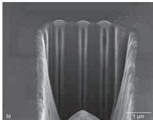
**Fig. 2:** a) PhC power splitter (EBL/ICP-RIE) with and without central hole (inset), b) FIB fabricated central hole with offset, funnel shape (left inset), redeposition (right inset/dashed circle).
