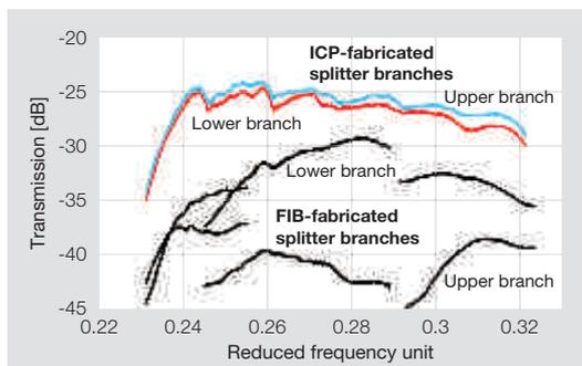
**Fig. 3:** Comparison of transmission: EBL/ICP-RIE only (grey), FIB-milled central hole with offset (black). Smoothed graphs to eliminate Fabry-Perot fringes (facet to facet cavity).
