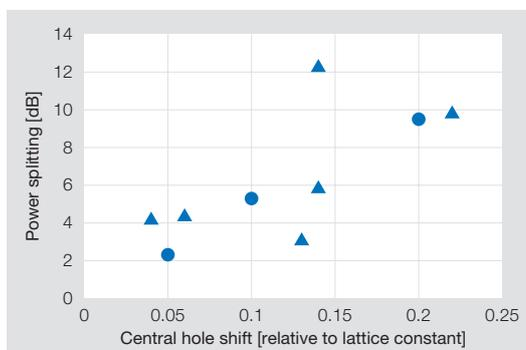
**Fig. 4:** Power splitting versus central hole shift: theory (circles), measurements (triangles).
