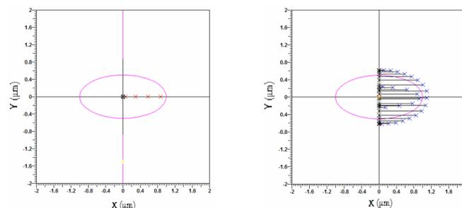
Excitation is plane wave. The boundary (ellipse, circle) in xy plane is defined. 2D multipole expansions is set in a half of the shape, due to a symmetry. 3D shape is defined by rotate the 2D one. 3D ring multipoles is generated.
